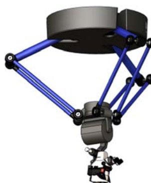
FIGURE 4.2 – SurgiScope (ISIS), porte-microscope à architecture Delta
