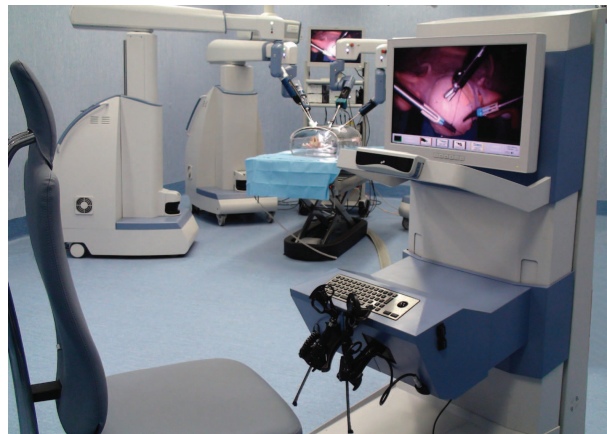
(a) The clinical prototype of the Advanced Laparoscopy through Force refleCT(X)ion (ALF-X) Teleap system. (Image credit: Sofar S.p.A)
