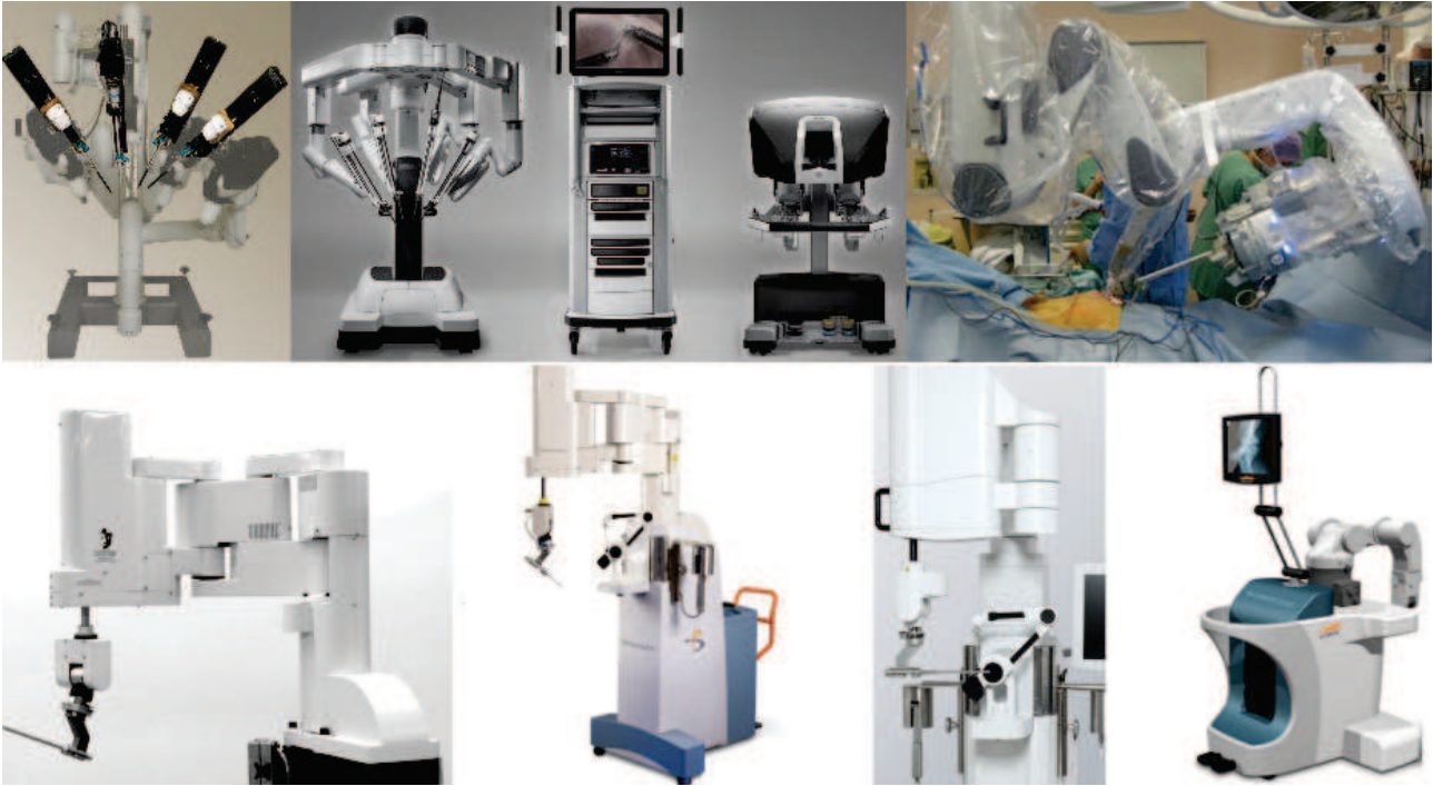
Figure 2. The two most famous surgical robots, Intuitive Surgical's da Vinci (top) and Curexo's ROBODOC (bottom) shown in their first commercial format (around 2000), current outfit and provisional future design. (Image credit: Intuitive Surgical Inc. (top row), ROBODOC , a Curexo Technology Company (bottom row)).
