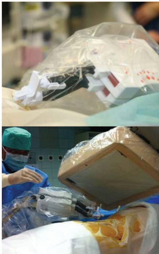
Figure 11. The iSYS mobile rack robot. The iSYS1 is a compact robotic targeting system to assist interventional radiology and neurosurgery procedures with 3D image-based needle path planning. (Image credit: iSYS Medizintechnik GmbH [143])
