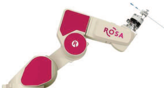
(b) The manipulator arm of the ROSA system. (Image credit: Medtech S.A.)
