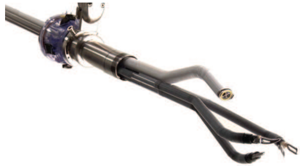
Figure 16. The da Vinci tool for single site surgery (image credit: Intuitive Surgical Inc.)
