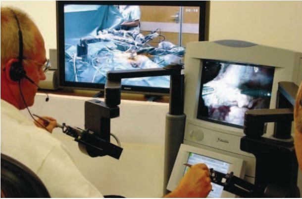
The Zeus robot pictured during the Lindbergh operation. The surgeon's console of the Zeus during the first transatlantic robot-assisted cholecystectomy in 2001 and the patient cart in Strasbourg (visible within the monitor). (Image credit: IRCAD.)
