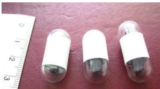
Figure 6. Camera capsules used for the internal examination of the oesophagus, the small intestine and the large intestine—from left to right. (Image credit: Dr. H.H. Krause, CC-BY-SA 3.0.)
