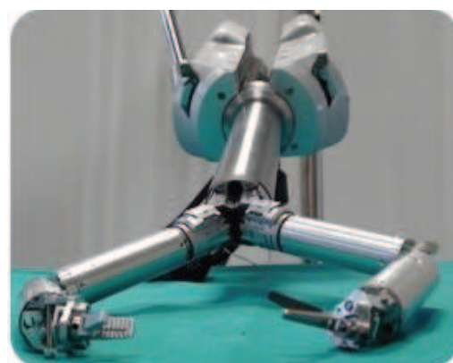
(b) The SRINT intra-abdominal robot. (Image credit: ARAKNES project and Scuola Superiore Sant'Anna.)
